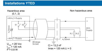
In area 0, the combination of the pressure switch and the safety barrier must be covered by a calculation checked by an approved body. For the application in Ex zone you have to respect the conditions mentioned in the ATEX Type Examination Certificate (LCIE 03 ATEX 6300 X). You find the certificates and manuals under http://www.baumer.com/
